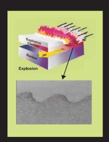
permanent, strong, crevice-free and leak proof metallurgical weld between dissimilar metals and alloys.
